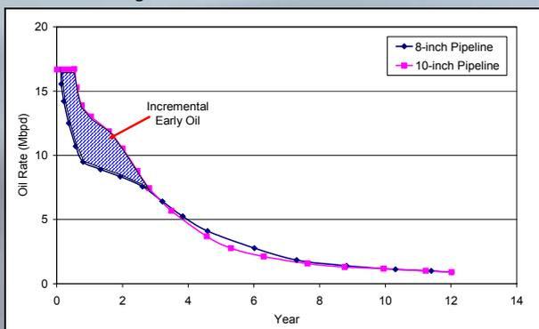
Figure 1 shows the effect of increasing the size of the pipeline transporting production from subsea wellheads to the host platform. Clearly the increase in pipeline size from 8 to 10-inch yields a significant improvement in early oil production and overall recovery.
